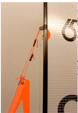
The first step in attaching the top of the jib is to attach the luff wire again I use dacron and attach in such a way that a downward motion on the bowsie tightens the rig the next is to attach the up haul from the top of the jib sail again attach in a way so that a downward motions tightens the rig.
