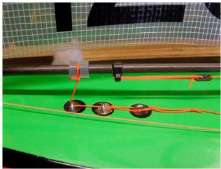
Again the boom attachment is attached to the Jib boom by forming a series of loops around the boom then tying a knot between 2 silicon bands, I then form a loop so that the boom sits about 20mm above the deck as per the DF instructions, I leave a tail on the end to help thread this cord through the deck eyes.
