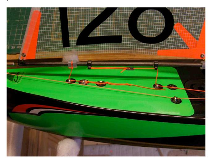
I go through deck eye 5 straight to the clip for the jib and just trough the deck eye to the clip for the main.
